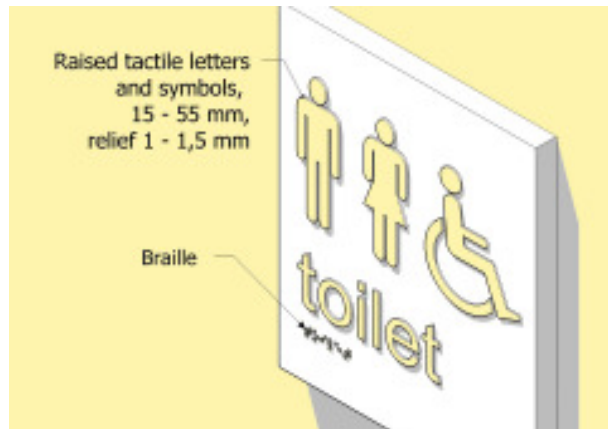
Figure 63 — Example of raised tactile signs and Braille
